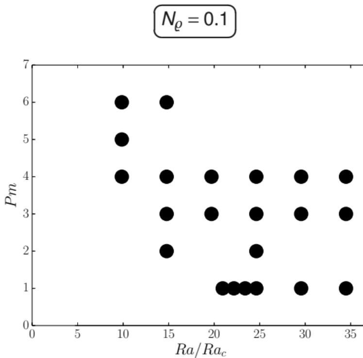
Dipolar dynamos as a function of  $Ra/Ra_c$  and  $Pm$
