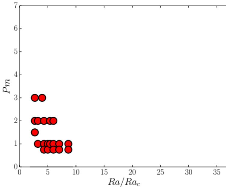
Dipolar dynamos as a function of  $Ra/Ra_c$  and  $Pm$
