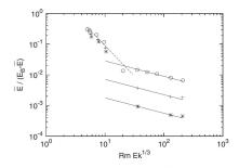
FIG. 5.  $\bar{E}/(E_B - \bar{E})$  as a function of Rm Ek<sup>1/3</sup> for A = 0.5 (circles), 1 (crosses), and 2 (stars). The dashed line follows the prediction of first order smoothing and shows  $\bar{E}/(E_B - \bar{E}) \propto (\text{Rm Ek}^{1/3})^{-2}$ . The solid lines plot the functions  $0.09/(\sqrt{x}, 0.09/(4\sqrt{x}))$ , and  $0.09/(16\sqrt{x})$ .
